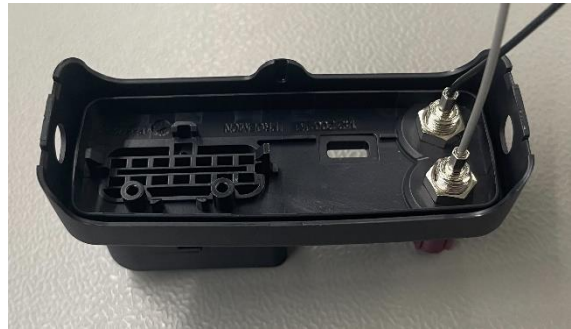
After: FAKRA connector without toothed washer
