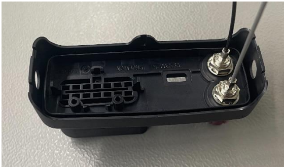
Before: FAKRA connector with toothed washer
